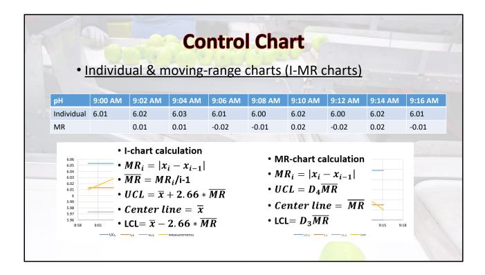
The table shows the measurements taken every two minutes continuously in a wash tank, and moving range is calculated between every two numbers. Once these values are calculated, equations listed here are used for calculating the UCL and LCL values for each chart. The D4 and D3 values are constant values that can be identified based on the degree of freedom. For the moving range chart, the degree of freedom is 2.
