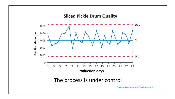
Here is the control chart built based on the number collected. You have UCL, CL, and LCL, and the percentage of defect of each production day shown on this figure and the process can be seen as under control.
