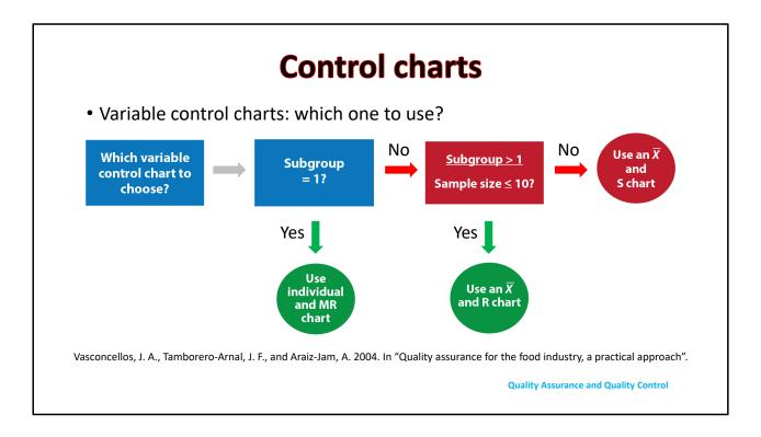
Here's a quick summary of the three sets of control charts. When measurements can be taken continuously, the set of individual and moving range charts is the best fit. This is also considered only one subgroup. When subsamples are taken at each sampling point and the number of samples taken at each time point is less than 10, the X bar and Range charts are a good fit. If more than 10 samples are taken at each time point, X bar and S charts are better to reflect the changes and variations.
