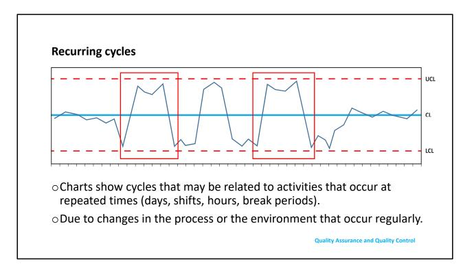
This chart shows a pattern called recurring cycles. These two identical curves might be caused by activities that occur at repeated times. Finding the root cause is again the key to preventing reoccurrence of the pattern.
