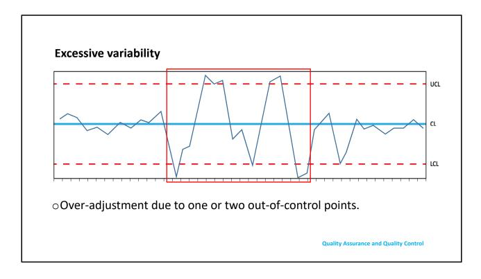
This is caused by over-adjustment of the system due to the overreacting to a couple of wild outliers. Identifying the root cause before adjust the processing line is important to avoid additional problems.
