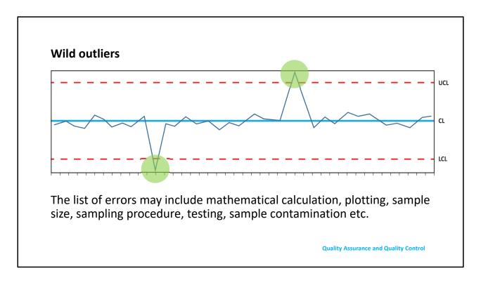
"Wild outlier" is another scenario. The list of errors causing a chart that looks like this might include mathematical calculation, plotting mistakes, sampling size mistakes, or testing errors. Do not overreact when an outlier is seen. Overreaction to an outlier problem might lead to the next chart, which we call excessive variability.
