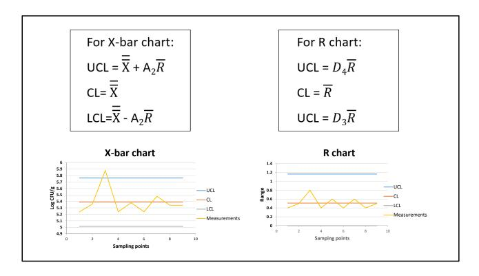
Similar equations are used for calculating the UCL, CL, and LCL values. The A2, D4, and D3 values are constant values determined by the degree of freedom. The degree of freedom for this example is 3. As four samples were taken, the degree of freedom is 4-1.
