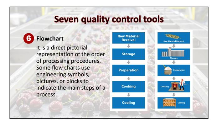
A flowchart is also a quality control tool. It is a direct pictorial representation of the order of processing procedures. Symbols or boxes with words can be used for establishing a flowchart. A flowchart is used as the first step for establishing a food safety plan or HACCP. A flowchart allows us to go over the entire process and identify steps at which control measures can be implemented and verified.
