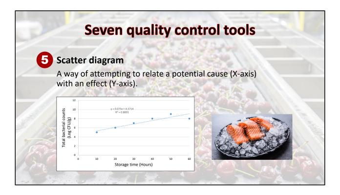
The fifth quality control tool is a scatter diagram. It is a way to present data and identify potential correlations between the causes and effects. The example given here shows the correlation between the total bacterial counts of a raw salmon product and storage time. As the storage time increases, the total bacterial counts increase. The regression line indicates quite strong correlations between the two.
