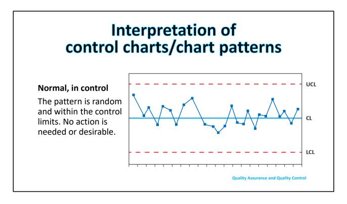
Once the control charts are built, the next step is to look at the charts and determine whether there are some potential problems within the processing line. We do expect that variance will happen, as shown in this figure. All values are between UCL and LCL, so this figure indicates that the process is under control and is normal.
