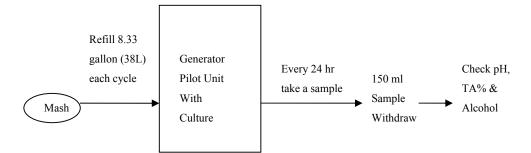
Figure 28: Generator Pilot Unit Flow Chart
