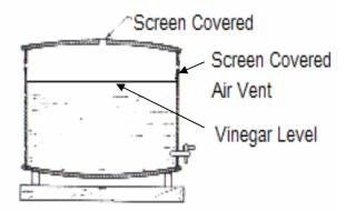
Figure 6: Orleans Process Barrel
