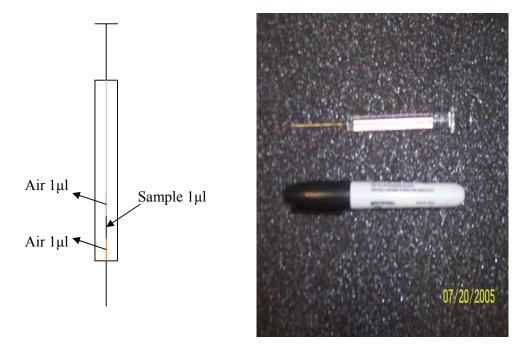
Figure 56: Injector Method
