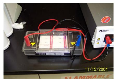
Figure 63: Electrophoresis Tray
