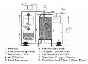
Figure 10: Semi-Continuous Process
