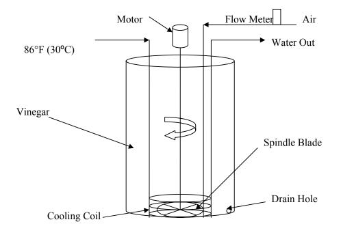
Figure 46: Diagram of Submerged Fermentor
