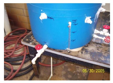
Figure 27: Drain Hose for Sampling
