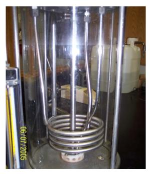
Figure 39: Cooling Coil in the Fermentor
