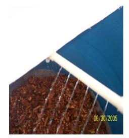
Figure 18: Liquid Sprays on Top of Chips
