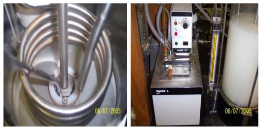
Figure 40: Cooling Coil Sit Above the Aerator Figure 41: Cooling Temperature Control
