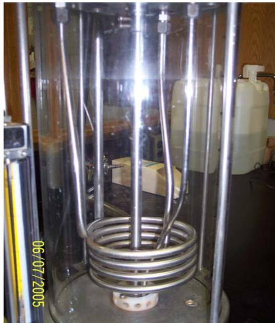
Figure 39: Cooling Coil in the Fermentor
