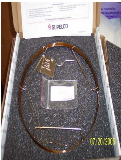
Figure 52: Capillary Column SPB-1000
