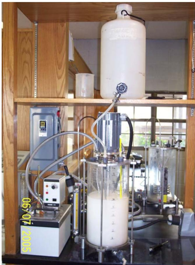
Figure 38: 9L Creole Lab Scale Fermentor
