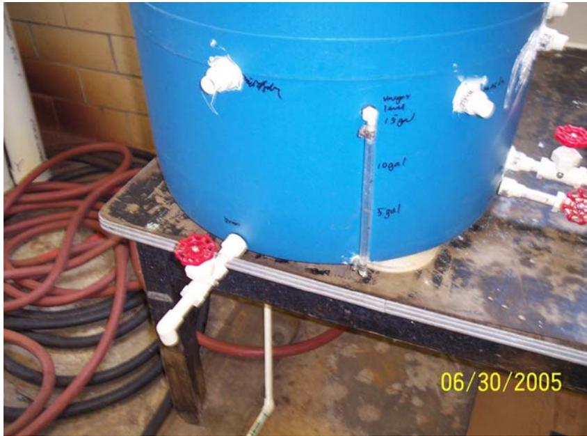
Figure 27: Drain Hose for Sampling
