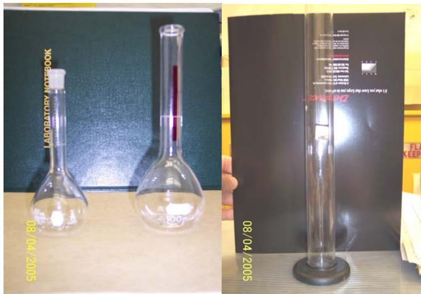
Figure 47: 50ml and 100ml Volumetric Flask and 200ml Cylinder
