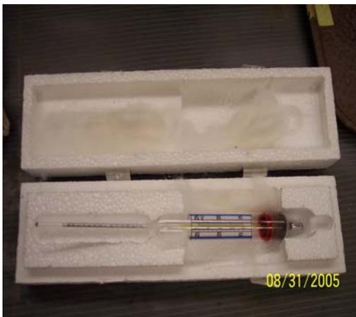
Figure 49: Alcohol Hydrometer
