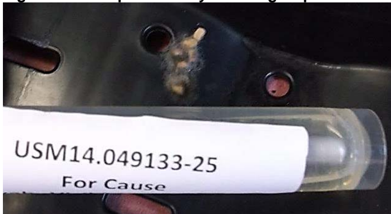
Figure 4. Example of decay and fungal sporulation in an RPC unit
