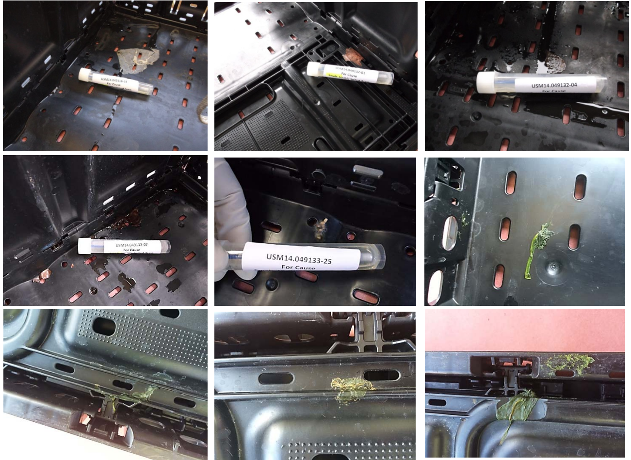
Figure 4. Example of decay and fungal sporulation in an RPC unit
