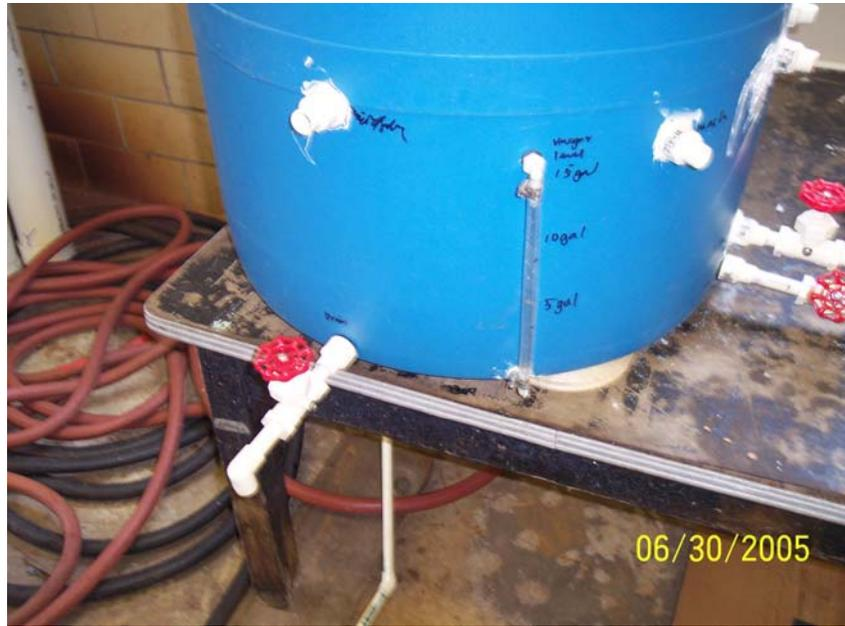
Figure 27: Drain Hose for Sampling
