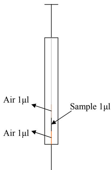
Figure 56: Injector Method
