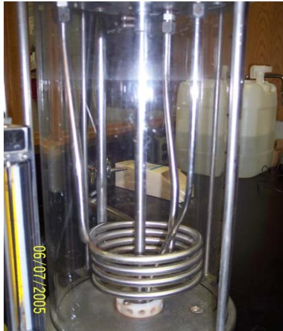
Figure 39: Cooling Coil in the Fermentor
