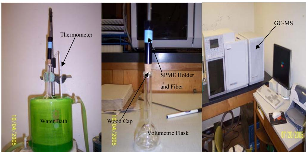
Figure 59: Water bath, SPME setup and GC-MS
