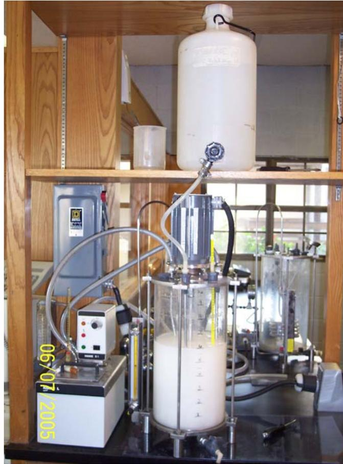
Figure 38: 9L Creole Lab Scale Fermentor
