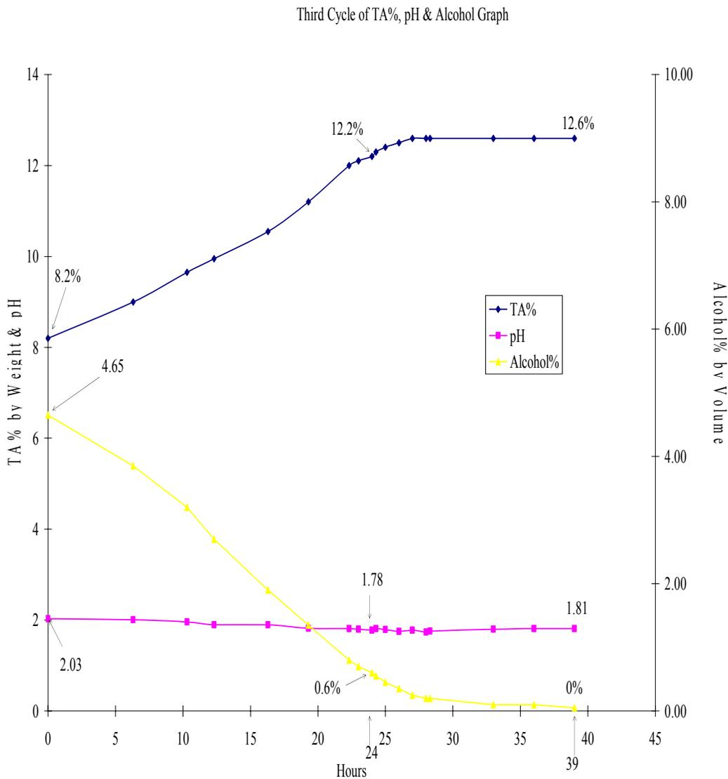
Figure 72: Third and Final Cycle – Submerged Process
