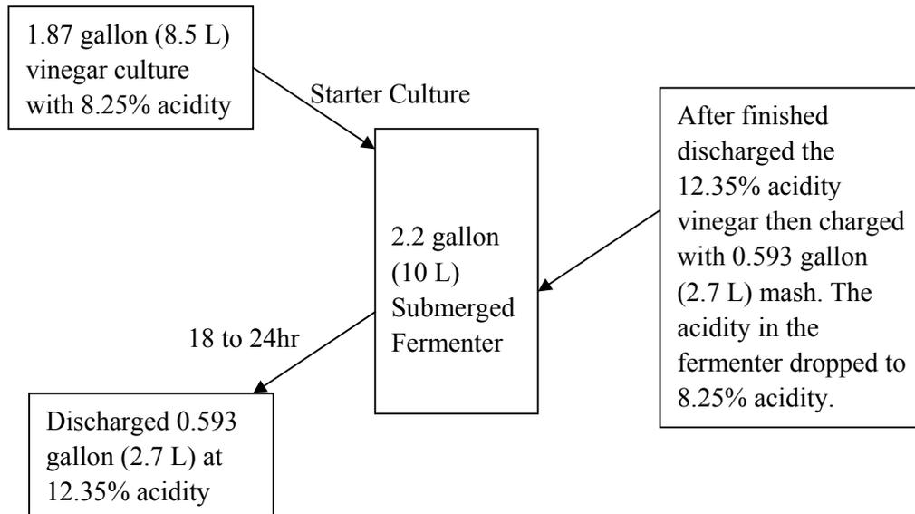
Figure 45: Submerged Acetification Process 2 Flow Chart
