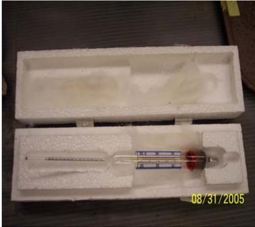
Figure 49: Alcohol Hydrometer
