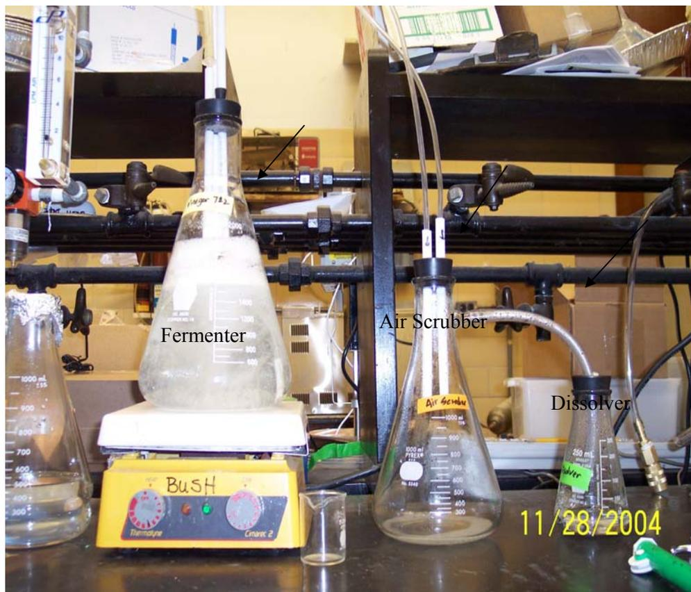
Figure 33: Submerged Processes 1
