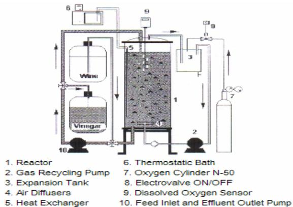
Figure 10: Semi-Continuous Process
