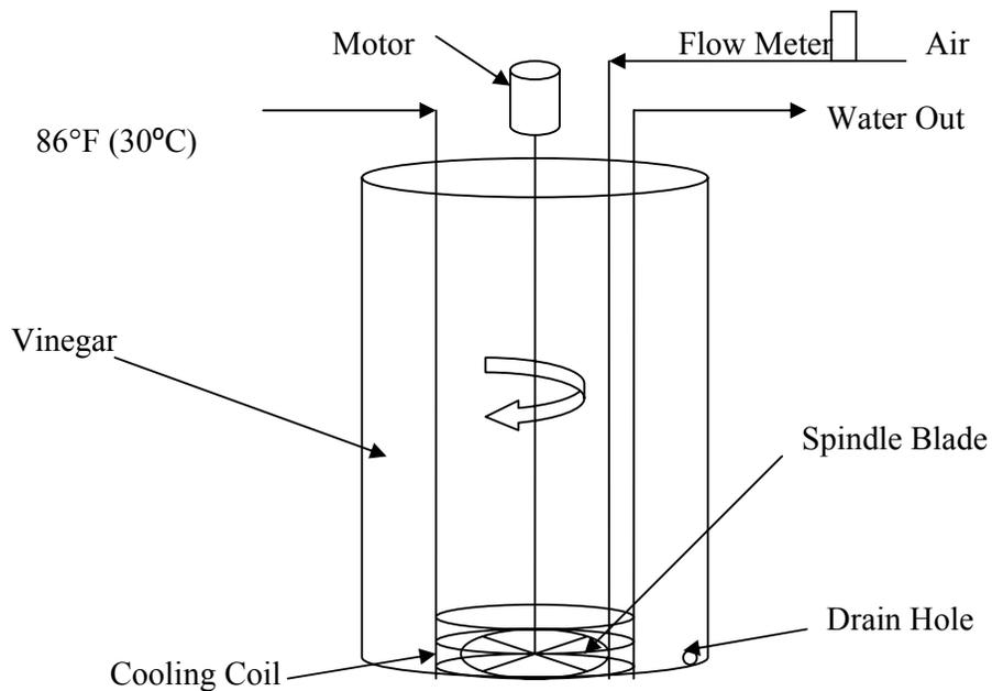
Figure 46: Diagram of Submerged Fermentor
