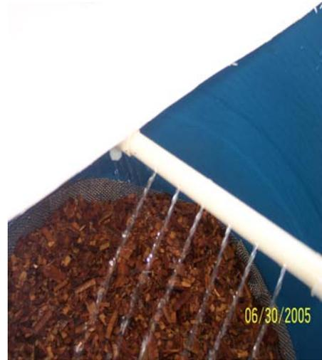
Figure 18: Liquid Sprays on Top of Chips
